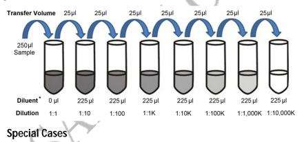
Serum and plasma typically require a 10,000-fold dilution in order for their OD readings to fall within the Standard Curve of this assay. However, due to sample variation, it is recommended that researchers determine the optimal dilution for their samples as described above.
