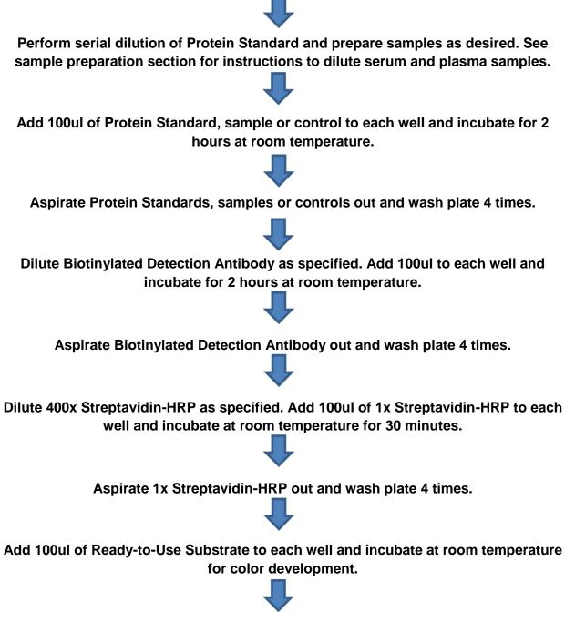
Add 100ul of Stop Solution and read plate at 450nm.
